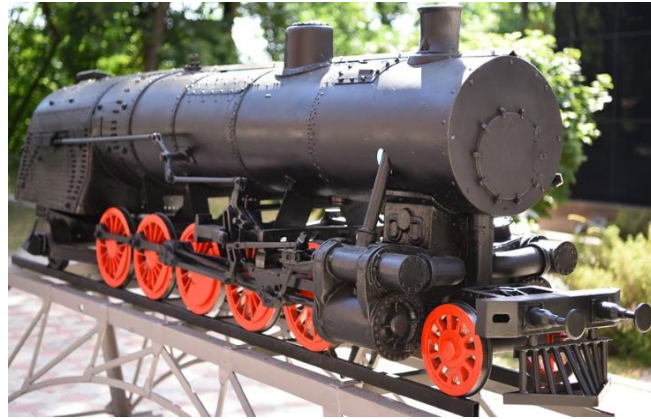
Fig. 2. Model of a steam locomotive with a 1-5-0 wheel arrangement, made at Kharkiv Mechanical Engineering Institute under the supervision of P.M. Mukhachov. Photo by M. Zaveriushchenko
